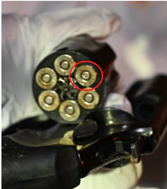
Image 4: A crime scene photograph of the open chamber of Muse's revolver on the night of the incident. The dented primer (circled in red) is indicative of a fired round.
